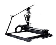
The Tactograph is a printer that was developed to produce tactile images from saved pictures. The basic design was developed through the Center for Rehabilitation Engineering and Assistive Technologies (CREATE) at IIT Madras, with constant feedback from end users and educators. Enability Foundation handles the marketing and commercialisation of the Tactograph. The challenge given to Enability in this study was to create a tactile version of the
